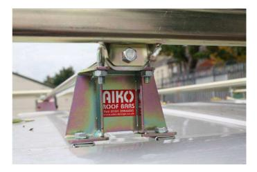
By now you should have the whole rack fully built up but still loose on the brackets, so now you can get everything sat equally across your roof and finally fully tighten the M8 Nylocs on all of the U-bolts. Stop tightening these as the bars are nipped; if you bend up the corners of the brackets at all, you've gone way too far- so aim for no more than 10nm torque.
